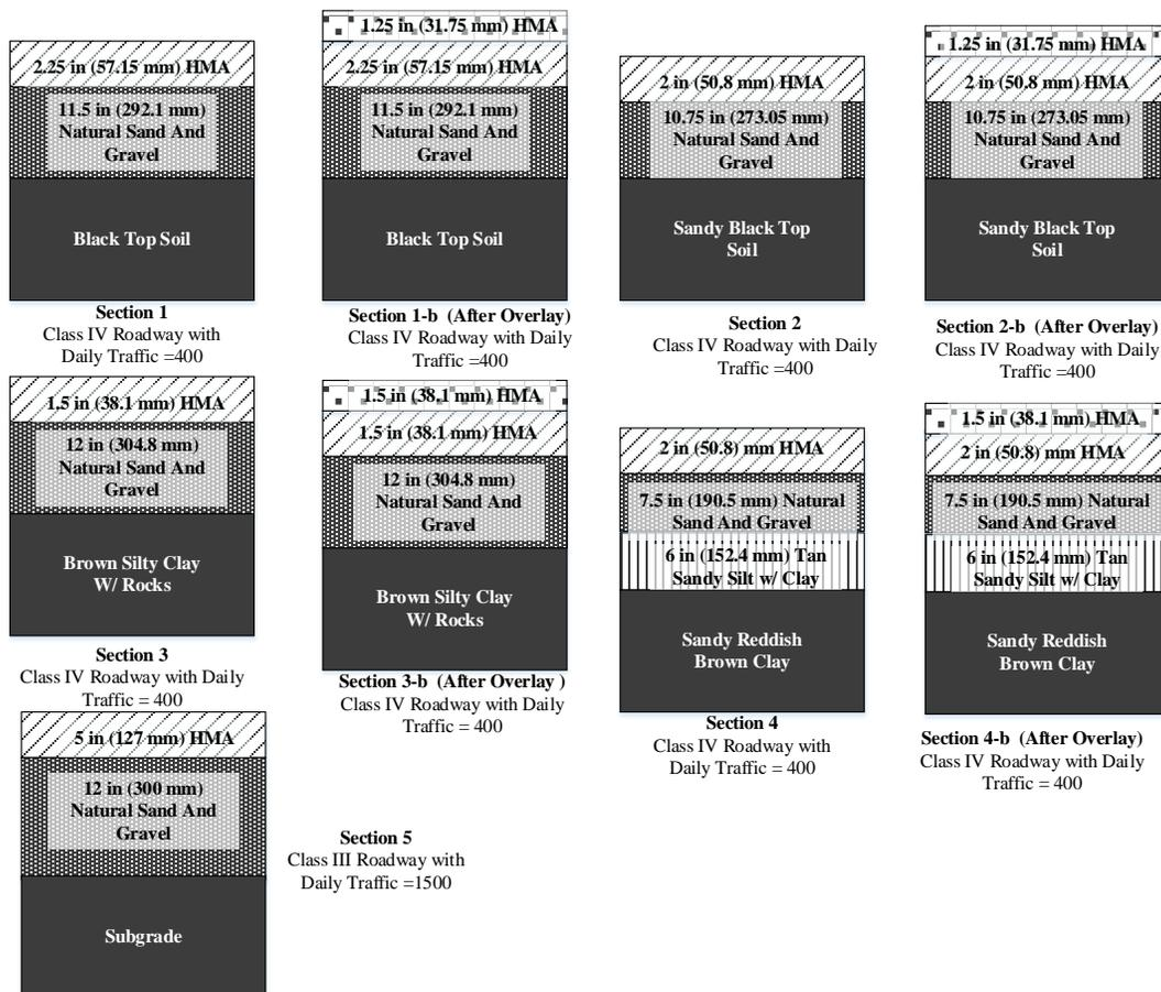
Figure 3.2: Layer Configurations and Traffic Information for Pavement Sections Selected for Current Study
