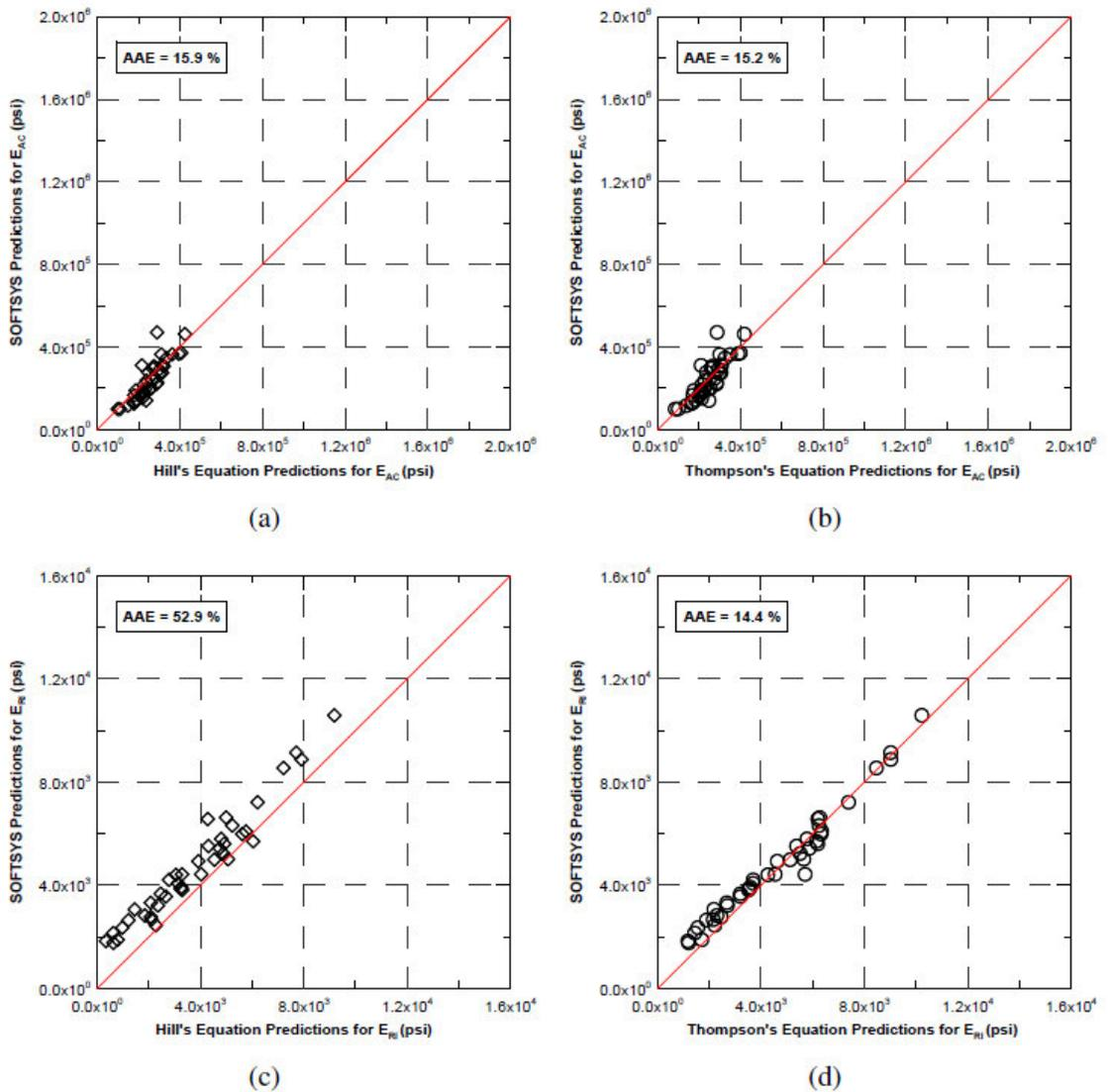
Figure 2.12: Performances of a SOFTSYS Model FDP-PM1-FWD4 for US 50 (Pekcan 2011)
