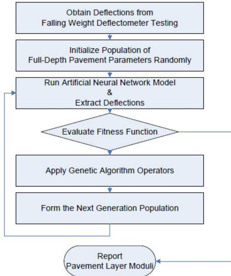
Figure 2.6: SOFTSYS Algorithm Flowchart (Pekcan et al. 2009)
