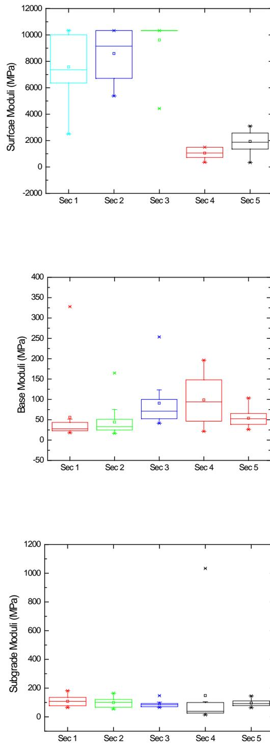
Figure 3.5: Back-Calculated Layer Modulus Values for Different Pavement Sections
