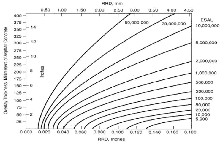
Figure 2.19: Asphalt Concrete Overlay Thickness Required to Reduce Pavement Deflections to Representative Rebound Deflection Value (AI 1996)
