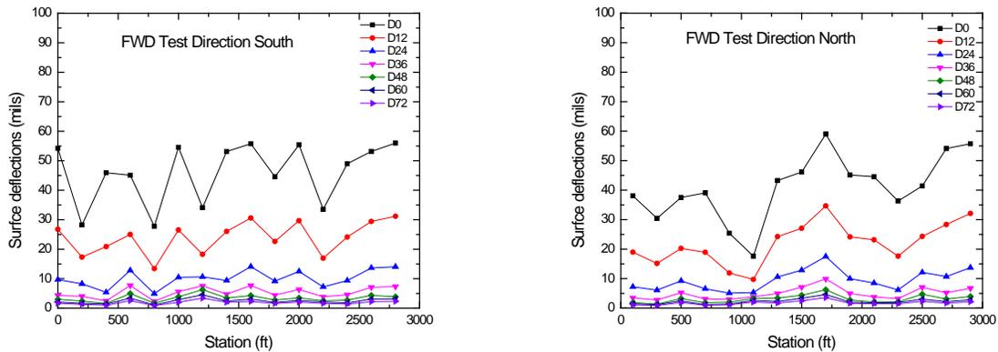
Figure 3.4: Deflection Basins Obtained from the Field during (a) Set 1, b) Set 2, and c) Set 3 FWD Testing Efforts for Pavement Section 2
