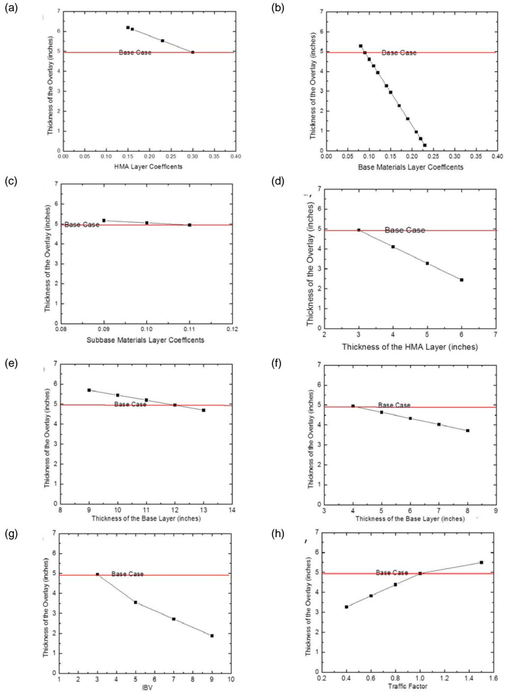
Figure 2.15: Overlay Thicknesses Calculated for Various Cases Studied as Listed in Table 2.4
