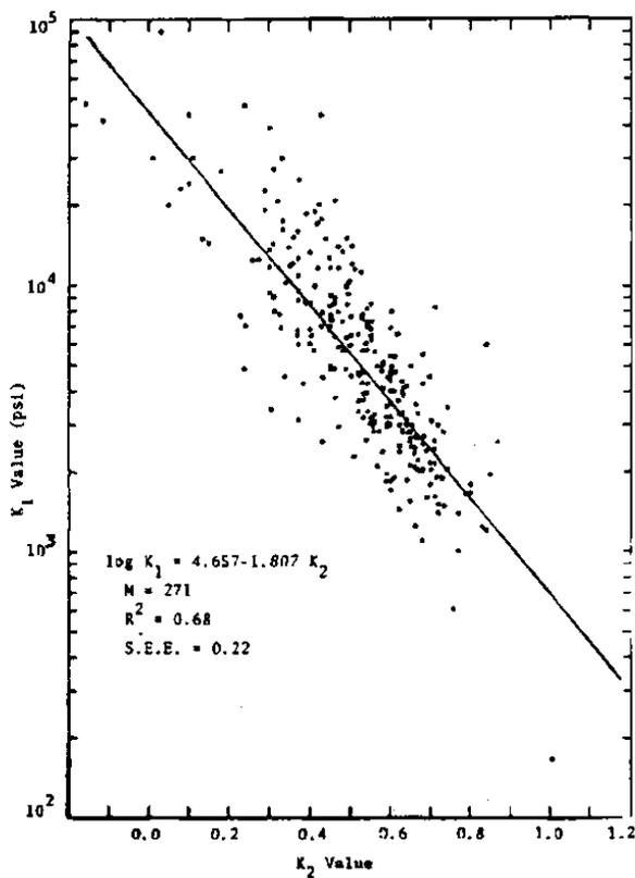
Figure 2.11: Relationship between K (shown as  $K_1$ ) and n (shown as  $K_2$ ) Values for Granular Materials Identified by Rada and Witczak (1981)
