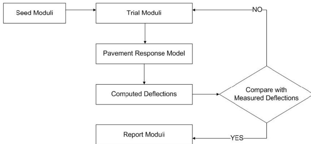
Figure 2.4: Traditional Iterative Backcalculation Procedure (Meier 1995)
