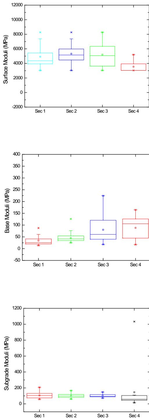
Figure 3.6: Back-Calculated Layer Modulus Values for Different Pavement Sections after Application of Overlay
