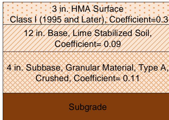
Figure 2.14: Pavement Layer Configuration Used as a Base Case
