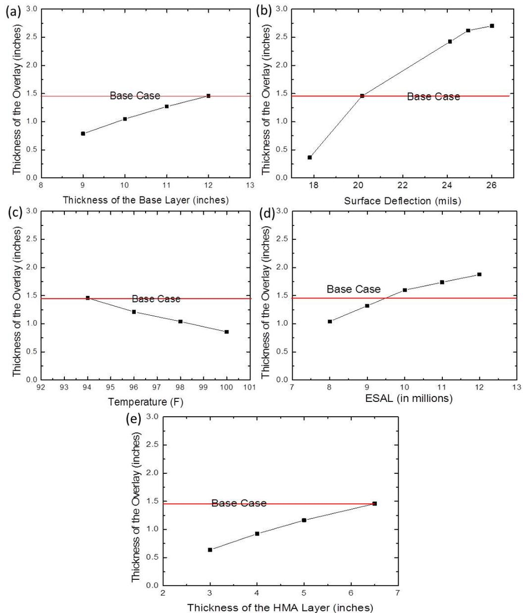
Figure 2.17: Overlay Thicknesses Calculated for Various Cases Listed in Table 2.6
