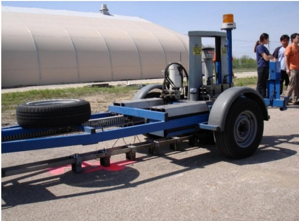
Figure 2.1: Dynatest Falling Weight Deflectometer (FWD) device at the University of Illinois
