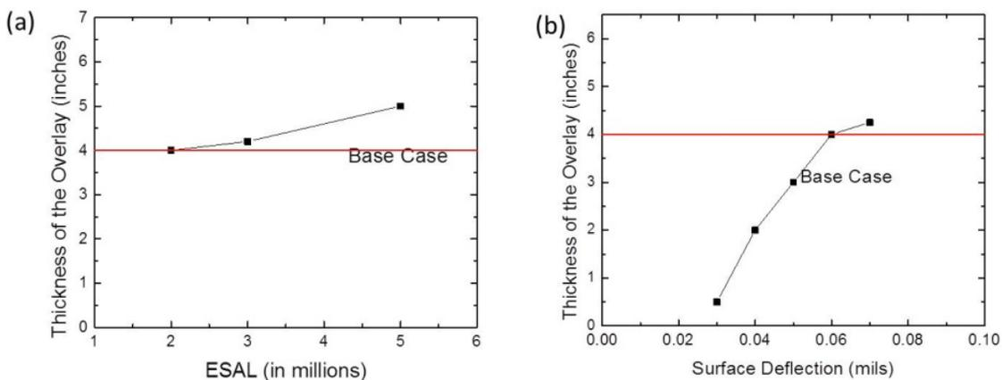
Figure 2.20: Calculated Overlay Thicknesses for the AI Deflection Method
