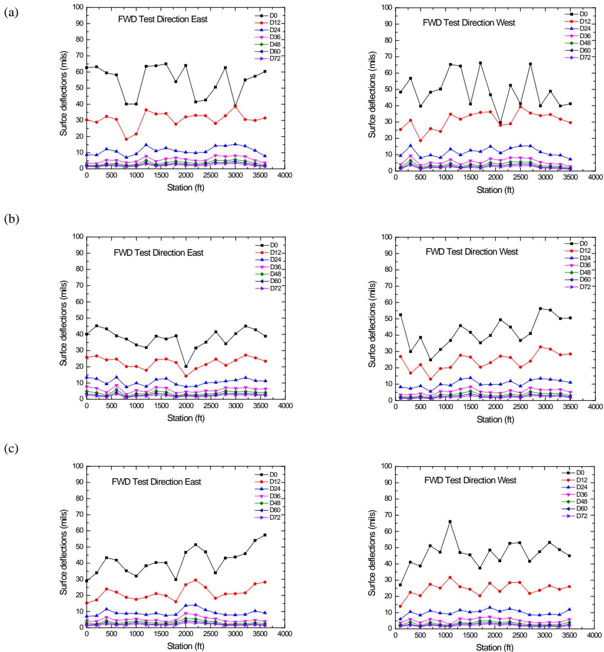
Figure 3.3: Deflection Basins Obtained from the Field during (a) Set 1, (b) Set 2, and (c) Set 3 FWD Testing Efforts for Pavement Section 1
