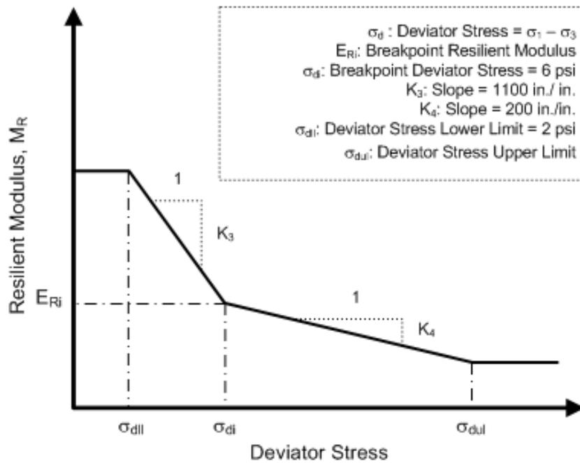
Figure 2.10: Bilinear Model to Characterize Stress Dependency of Fine-Grained Soils
