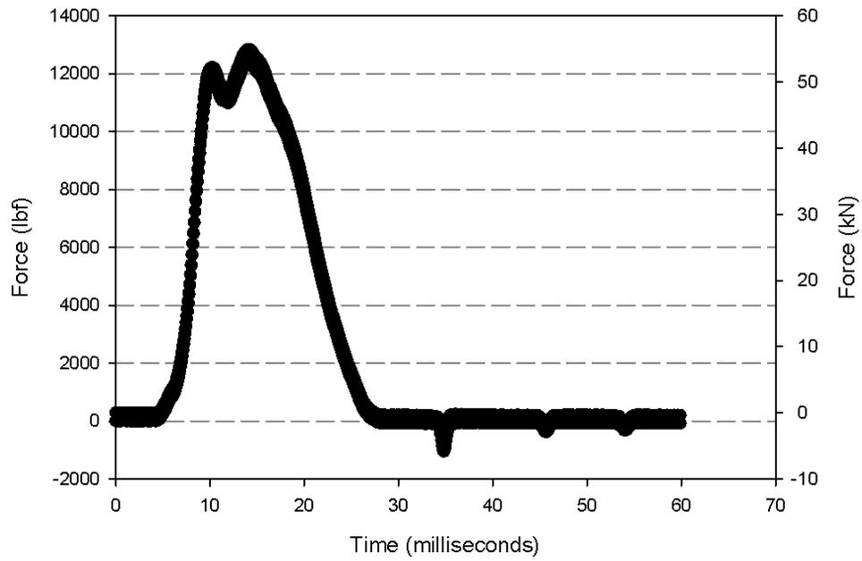
Figure 2.2: Haversine Loading Applied by FWD device
