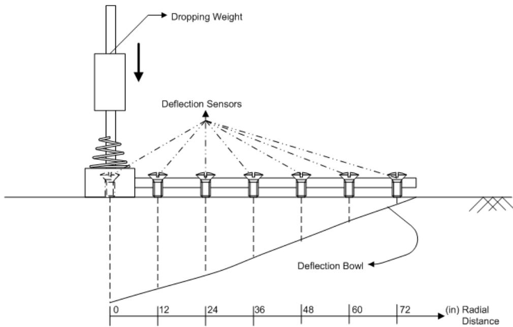
Figure 2.3: Locations of FWD Sensors and Schematic Drawing
