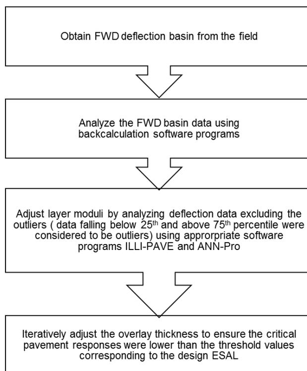
Figure 3.8: Flow Chart of the Developed M-E Overlay Design Procedure
