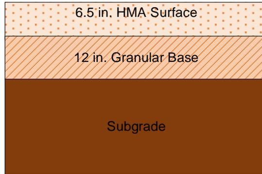
Figure 2.16: Pavement Layer Configuration Used as a Base Case
